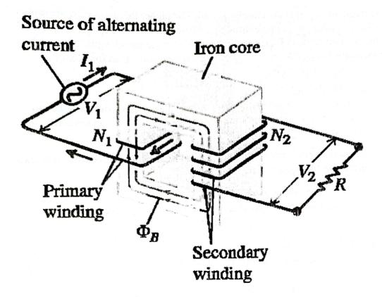
A transformer is an electrical device used to change a given alternating emf into a larger or smaller alternating emf.
