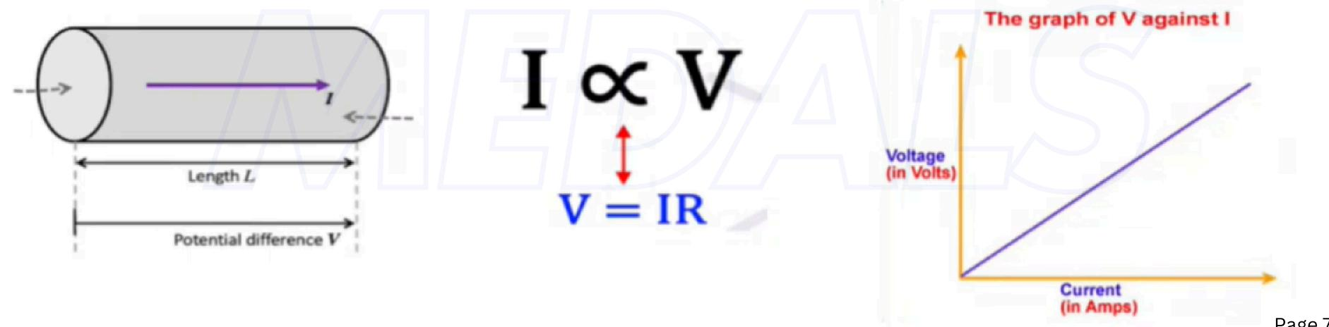
R = Resistance of conductor (Constant for ohimic conductor).
