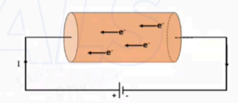
• One Ampere current :- one coulomb charge flow through a wire in one second.
