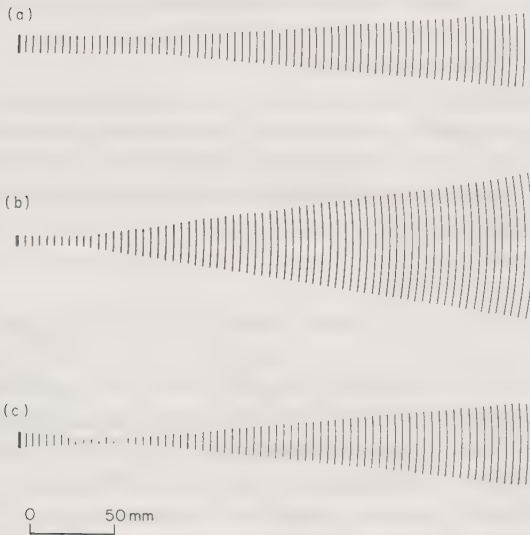
Fig. 19.2 Diagrammatic representation of the approximate shape of ultrasonic beams in water. Frequency f = 3 MHz; velocity c = 1\,500 m s -1 ; wavelength \lambda = 0.5 mm. Transducer diameter: (a) 10 mm unfocused; (b) 5 mm unfocused; (c) 10 mm focused.
